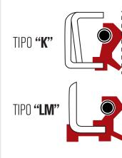
Reinforced structure design offer better protection for the area of the sealing lip.
